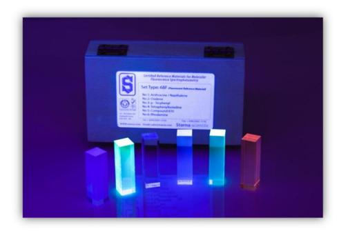
Consists of six polymer blocks containing seven fluorescent compounds whose spectra cover a broad spectral range with emission maxima from 330 to 582nm and excitation maxima from 290 to 562 nm. This wide spectral range enables the user to select a reference material with broadly similar spectral properties to those of the analyte, ensuring a reasonable spectral overlap and measurable signals without changing important parameters such as slit widths and wavelength settings.
